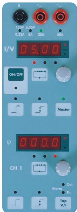
Current / voltage channel
